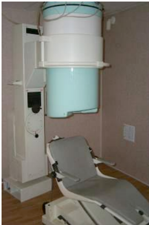
Figure 11. The 165-channel MEG system installed at ITAB, University of Chieti.
